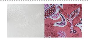
Jacquard fabrics exposed for high-grade and tasteful, but the richer the color, the higher the production cost. The "jacquard printing" double-sided printing process can simulate multi-color jacquard effects on white jacquard fabrics, reducing the production cost of jacquard fabrics.
